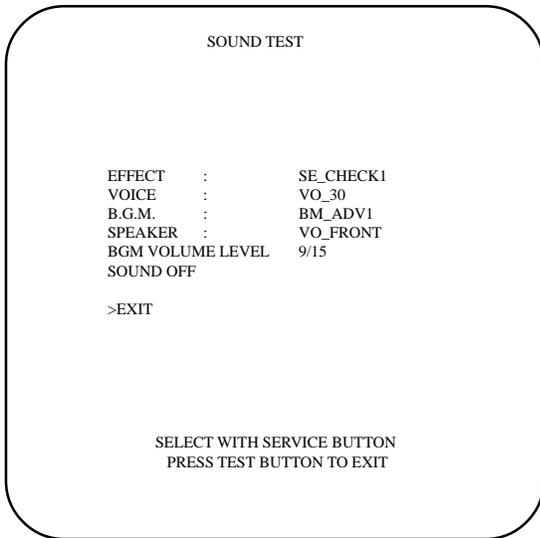
In the TEST mode, selecting SOUND TEST causes the screen, on which sound related BD and wiring connections are tested, to be displayed. be sure to check if the sound is satisfactorily emitted from each of speaker and the sound volume is appropriate.
