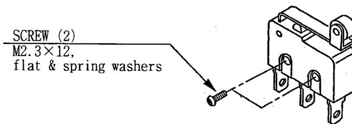
After replacing the Switch, check to see if the switch is inputted as per Shift Lever operation in the Test Mode.d
